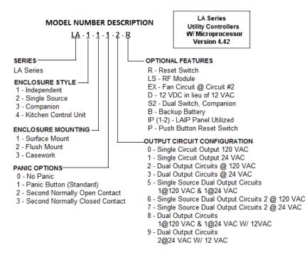
NOTE: Output Configurations 5, 6, 7, 8 and 9 are intended to operate with specific operators and solenoids for applications such as Instructor's Demonstration Stations and Science Preparation Rooms. When Configurations 2 or 3 are specified with Single Source Units, then Outputs are typically provided as single switch operators with or without a Reset per each output.
